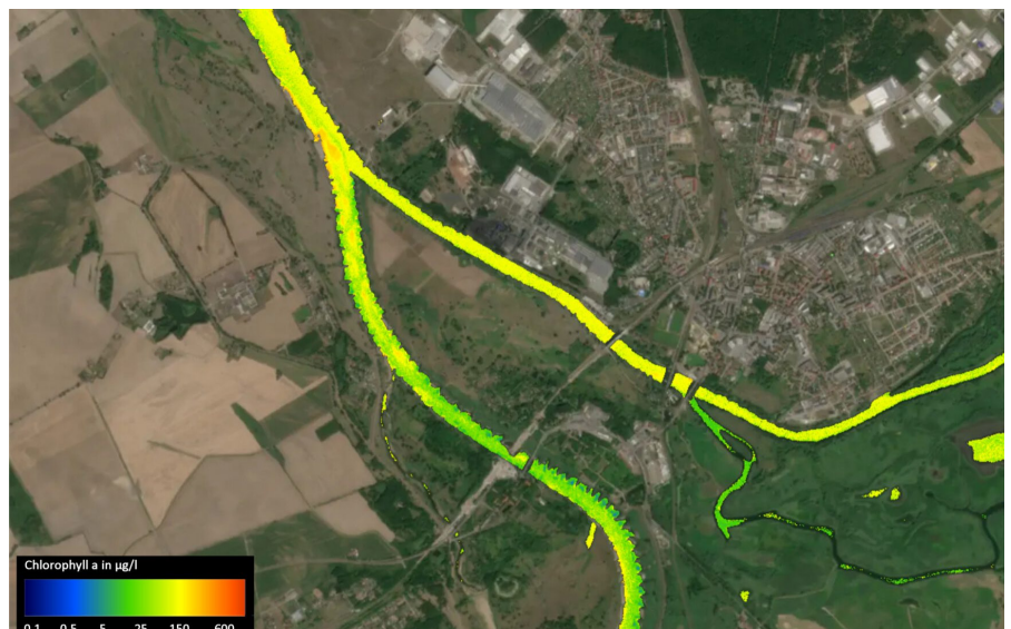
The image shows the inflow of the Warta (right) at August 3 2022, carrying markedly higher algae concentrations increasing the algal level in the Odra below significantly. c/ EOMAP / Planet https://www.eomap.com/press-release-satellite-data-reveals-details-of-oder-river-disaster/
